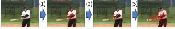
Figure 2. Steps to extract the ST feature. (1) detected SURF points, (2) detected SURF points with motion, and (3) obtained Delaunay triangles. (Cited from [24])
