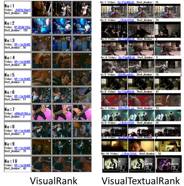
Figure 4: Diversity of results obtained by video shot retrieval system with VisualRank (right) and with VisualTextualRank (left). The category here is “play+guitar”. In the original framework [3], more than half of top 10 shots are from the same video with ID “6P-1e1QwRE” since they are visually similar. On the other hand, applying VisualTextualRank can select relevant shots from different videos since it regards not only visual similarities but also textual similarities of the shots.
