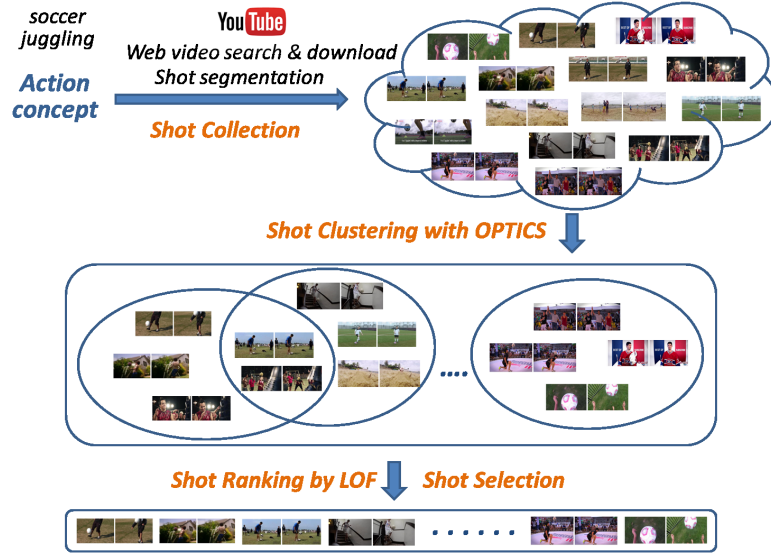
Fig. 1. Framework of our approach for automatic construction of action shot datasets which consists of three steps: shot collection, shot clustering and shot ranking.
