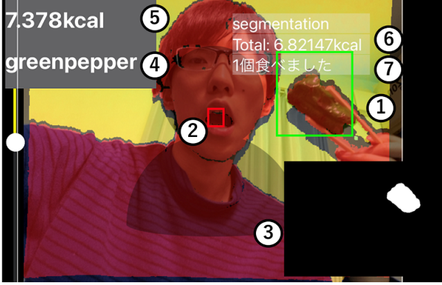
Figure 3: User interface of the proposed method (1. Food area bounding box, 2. Mouth area bounding box, 3. Food mask, 4. Detected food categories, 5. Estimated calorie content, 6. Total amount of calories currently taken, 7. Number of food instances currently taken)
