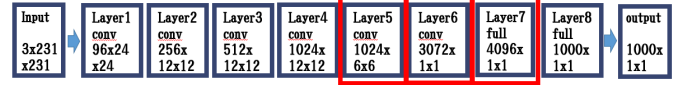
Fig. 2. The structure of the Deep Convolutional Neural Network (DCNN) for the ILSVRC 2013 dataset in Over feat[2]. We extracted feature vectors from the Layer-5, the Layer-6 and the Layer-7.
