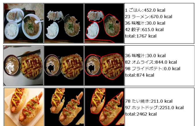
図9 凸包による食事領域の (1)original image , (2) segmentation result , (3)outline, (4)conv hull, (5)calory estimation
